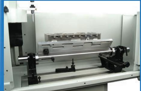
*RMC's optional quick mounting and leveling rolover fixture lets you surface most passenger car and medium size diesel heads and blocks.*
