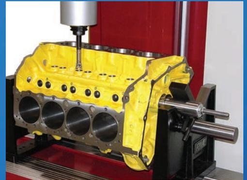
**More versatility!** RMC's Cylinder Boring Mills various fixtures attach quickly and easily to either the RMC 1000 or RMC 1550. They offer very cost effective method of boring and milling without the expensive cost of stand alone machines. Shown here with a Cummins NH block, the RMC-1550 Boring Mill can easily handle diesel blocks as large as the D8 Caterpillar.
