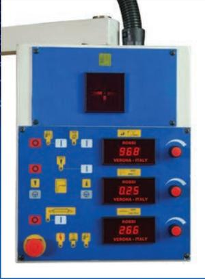
RMC Boring Mills have easy to read and use **control panels** as shown to the left with **RMC's exclusive digital bore centering display** on top. Also pictured is the optional 3-axis linear scale with digital read out below the control panel. To the right is a close up of RMC's adjustment for bore center which is faster than ever with RMC's digital bore centering feature.
