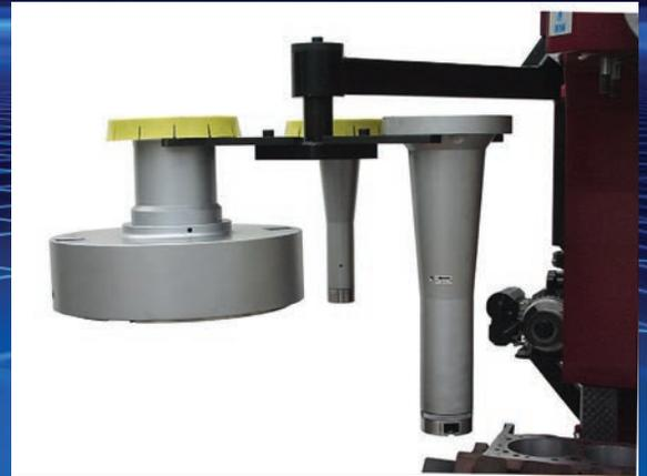
**RMC's heavy duty spindle caddy system** allows for faster setups and change over from boring to milling as well as providing convenient storage for three spindles.
