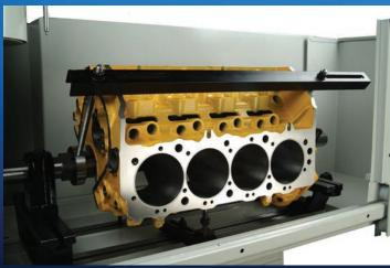
RMC's optional quick mounting rollover fixture lets you parallel deck both sides of the block without dismounting and resetting the block The fixture works with blocks up to 28" long and with cylinder heads up to 31" in length.
