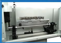
RMC's optional quick mounting and leveling rollover fixture lets you surface most passenger car and medium size diesel heads and blocks.
