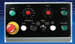
The RMC control panel is conveniently located and provides quick and easy access to all of the functions and operations on these surface milling machines. RMC's auto cycle function stops the table after the milling operation is complete, positions the tool to the front and returns the table to the start position without lifting the head.
