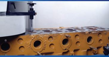
Surfacing the CAT 3406E with a standard touch off indicator
