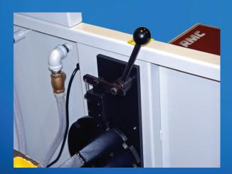
RMC's auto-centering fixture has been designed to make cylinder block setup easier and quicker than ever before. The drop down front doors give quick open access to work pieces for faster loading and unloading.
