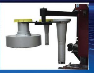
**RMC's heavy duty spindle caddy system** allows for faster setups and change over from boring to milling as well as providing convenient storage for three spindles.
