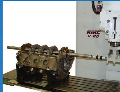
Center 3 Main Conversion setup, bar runs in bushings front and rear, no end plates needed.
