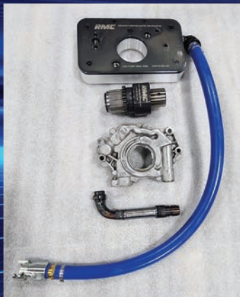
Pump Test Fixture Chrys 5.7 Hemi
