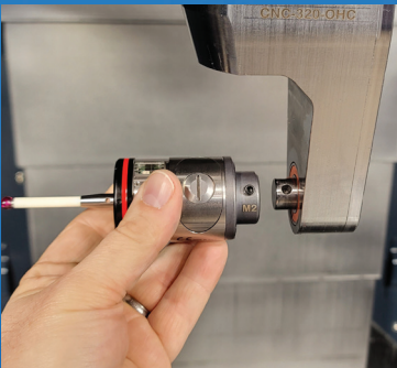
Rmc V35 probe install.
